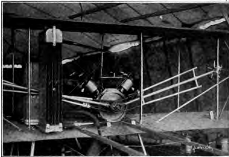
Fig. 10. Complete Power Plant and Transmission of Wright "Baby" Biplane
